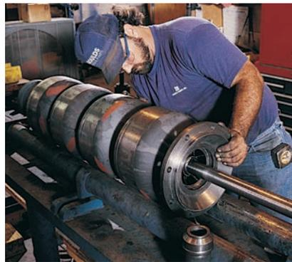
Our modern manufacturing facilities assure dimensionally consistent, high quality, fully machined parts, produced on a volume basis to bring down costs. Every impeller is precision balanced on a micro processor balance analyzer. Bell & Gossett is one of the largest manufacturers in the turbine industry.
